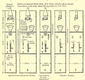
Note: Panels over 4000 Amp. have Top Sections 40 In. High and for Fig. A. and C. are 20 In. Wide. Generator and Converter Panels 4,000 Amp. and Less for Installation in the Same Board with Larger Panels will also be Furnished with 40 In. Top Sections.
